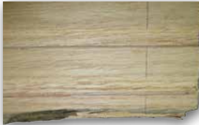
Bottom of Board Defect
